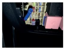
4. Insert fuse jumper into fuse box.
