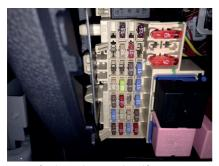
2. Open fuse box and remove selected fuse.
