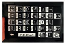
1. Identify ignition (+) fuse circuit i.e. radio. DO NOT connect to any primary vehicle safety systems.
